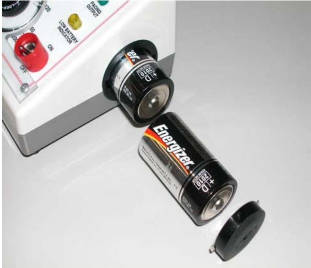
Turn POWER switch to OFF position. Locate the battery compartment on the side of the TAPSYSTEM Model 2A. Open the compartment by turning the cover until metal plate is exposed or groove on tab is horizontal. Remove the cover. The batteries are oriented with + terminals facing the battery compartment cover. Verify polarity before inserting the batteries. Insert batteries and replace compartment cover.
