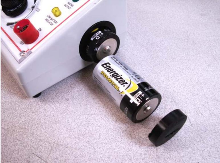
Turn POWER switch to OFF position. Locate the battery compartment on the side of the TAPSYSTEM Model 2A. Open the compartment by turning the cover until metal plate is exposed or groove on tab is horizontal. Remove the cover. The batteries are oriented with + terminals facing the battery compartment cover. Verify polarity before inserting the batteries. Insert batteries and replace compartment cover.
